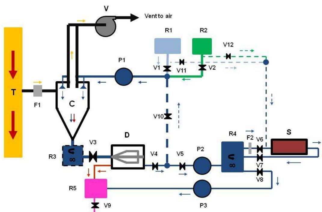
Figure 5. Mycohunt sampling system (option I, with cyclone). Parts signed with broken lines are optional. Abbreviations: T: Loading tube, F1, F2: filters: C: cyclone, V: ventilator, P1-P3: liquid pumps, R1: reservoir of solvent (water/acetonitrile), R2: reservoir for buffering agent (PBS), R3: Optional buffering and mixing reservoir, R4: Buffering and mixing reservoir, R5: waste reservoir, V1-V9 micro controlled valves, S: sensor.
