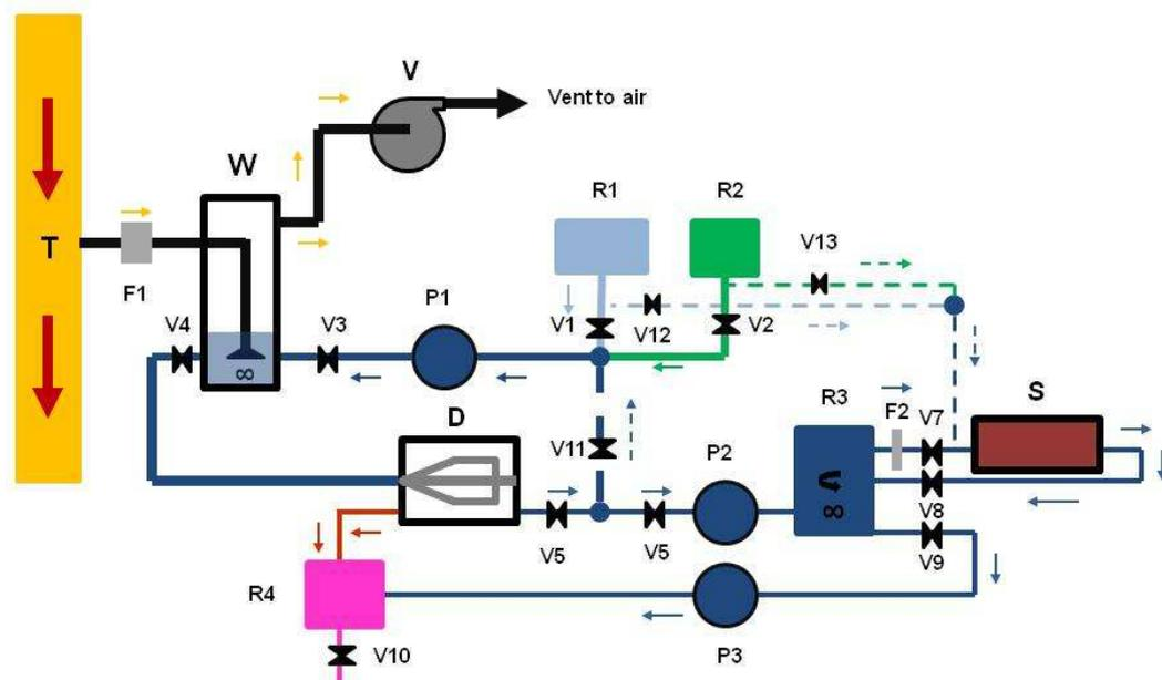
**Figure 6. Mycohunt sampling system (option II, with washing flask). Parts signed with broken are lines optional. Abbreviations: T: Loading tube, F1, F2: filters: W: washing falsk, V: ventilator, P1-P3: liquid pumps, R1: reservoir of solvent (water/acetonitrile), R2: reservoir for buffering agent (PBS), R4: Buffering and mixing reservoir, R4: waste reservoir, V1-V10 micro controlled valves, S: sensor.**
